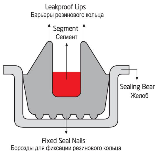
**NO LEAK WITH SEGMENT SEAL:**
